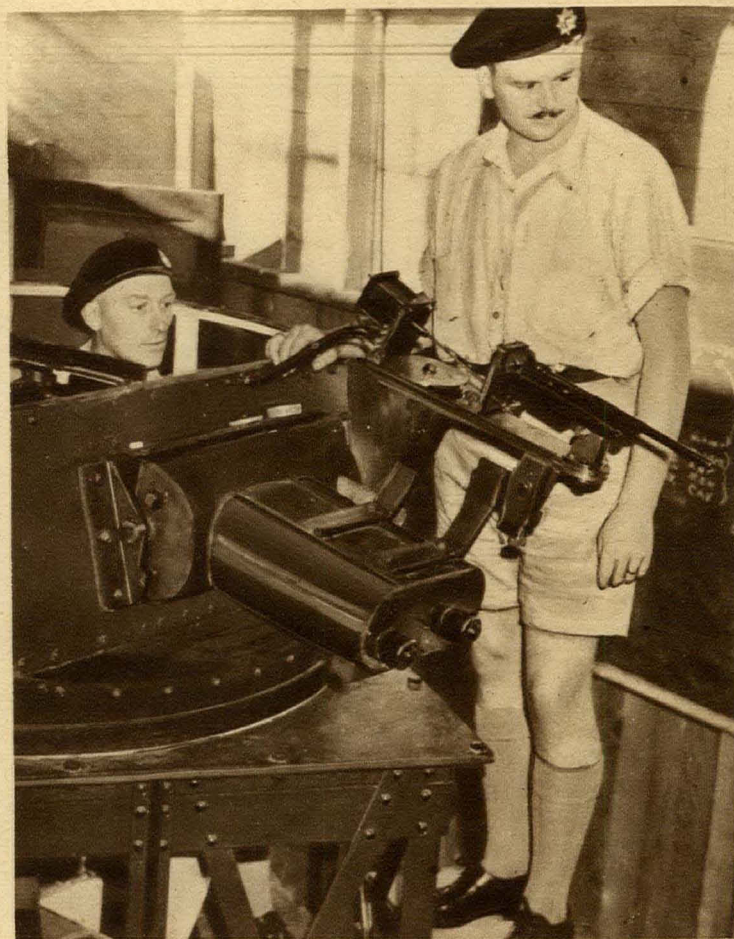
THIS "SCHOOLROOM TANK" at Camp Borden is an electrically driven dummy which jolts and rears, giving all sensations of the "real thing"
